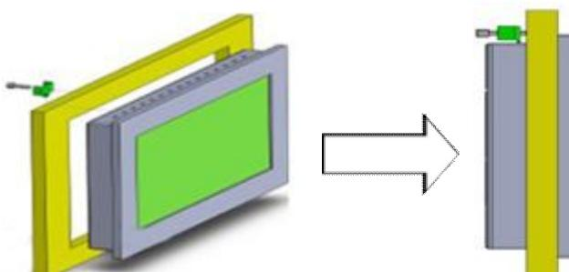
Put the unit through the panel cut out. Slide the clamps into the 4 holes provided around the case. Tighten the clamping screws in an even pattern until the unit is secured in the panel.
